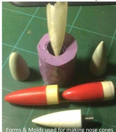
Forms & Molds used for making nose cones
