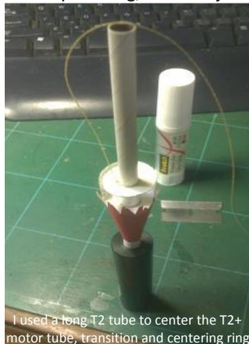
I used a long T2 tube to center the T2+ motor tube, transition and centering ring.
